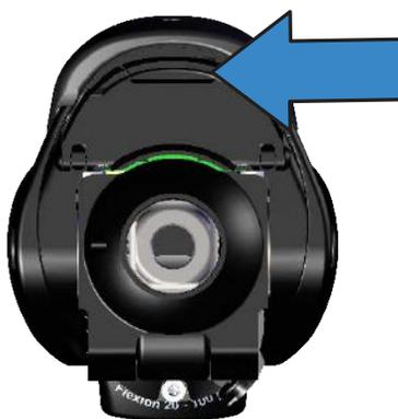
To Open: Press down latch. (The cap will spring open).
